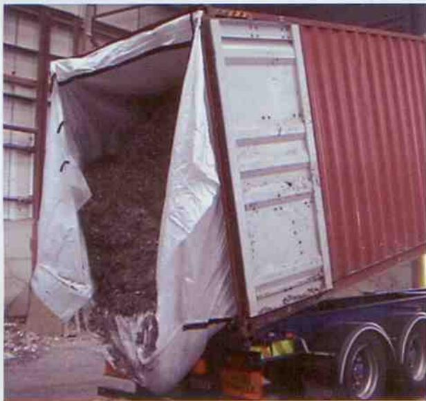
Figure 3. RDF unloading from 40 in. containers.
