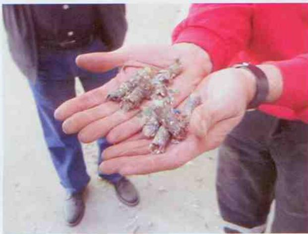
Figure 1. RDF hard pellets for bulk transport.
