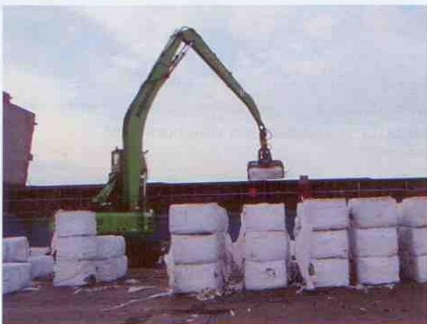
Figure 4. Loading vessel with RDF at MVW Lechtenberg's port facility in Germany.
