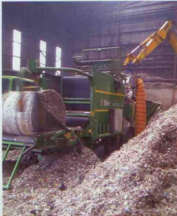
Figure 2. Baling and wrapping of RDF.
