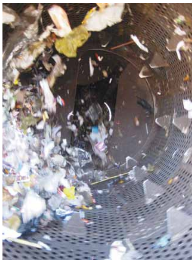
Figure 4. The view inside a drum screen for fines separation.
