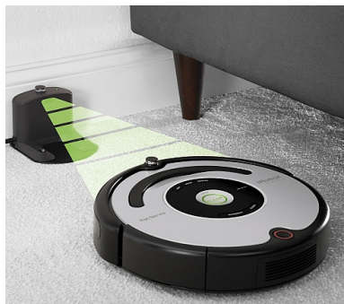
Figure 5-1: iRobot Roomba vacuum cleaning robot (iRobot 2011)
