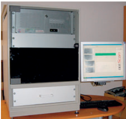
Figure 6: The braille inspection system DotScan
